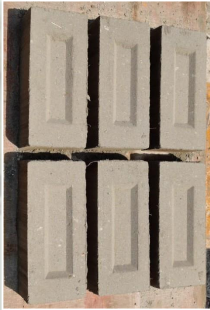
Bricks made from Salt Free Residue Ash
